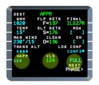
Note: Make sure CONF FULL is selected while adding the increment to VLS and setting it as VAPP because VLS for CONF 3 is higher than FULL Flaps CONF.
