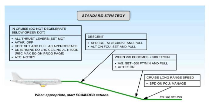
Note: Pressing the EO CLR key on the MCDU restores the all engine operative predictions and performance. Reverting to one engine-out performance again is not possible.
